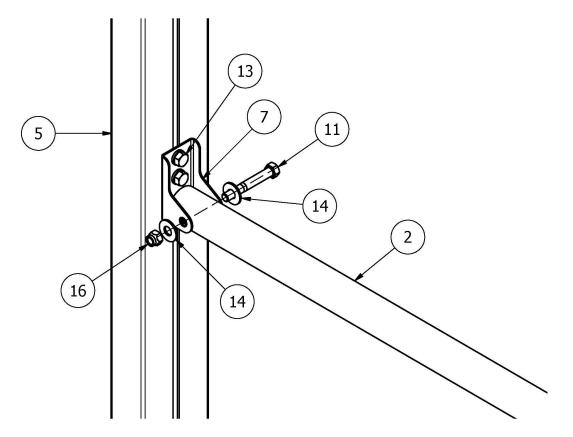
The bottom side of the backstay pipe should be 24" above the bottom of the Side Rail.
