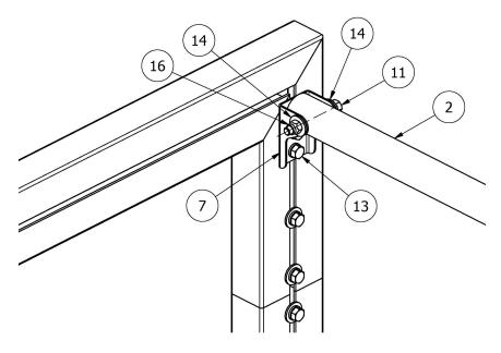
5) Attach the Backstay Brace Pipe (3) near the back of the two side backstay pipes. (see the following illustration). Use two Brace Clamp halves (8) to attach each end of the brace pipe. Insert a 5/16" x 2-1/2" carriage bolt (18) from the bottom as shown. Secure with a 5/16" flat washer (18) and a 5/16" nylon lock nut (20).
