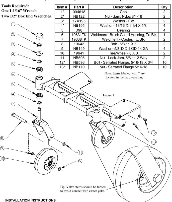
• Assemble the casters to the brush guard using the hardware from the hardware bag in the order shown in Figure 1. Using a 1-1/16" wrench, tighten item number 2 (NB122) enough to engage the nyloc portion of the nut while still allowing the caster to rotate freely. Item numbers 12 (NB596) and 13 (NB170) will be installed in a later step.
