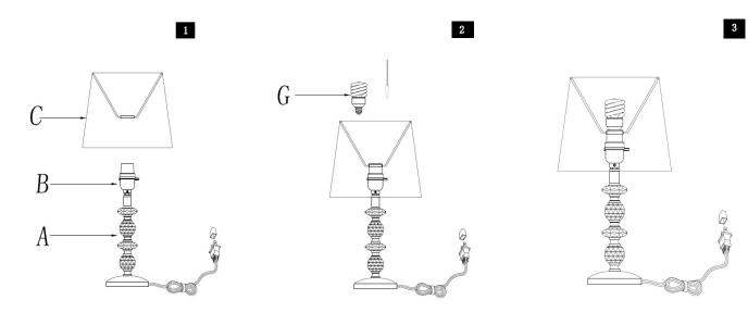
Step 1 Unpack all parts from cartons carefully Put the shade(C) on the Socket(B), then
