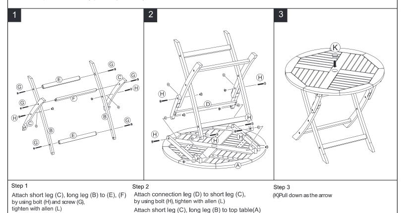
by using bolt (H), tighten with allen (L)
