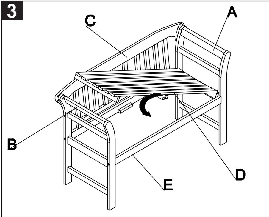
Step 3: put the seat (D) inside the bench as shown on the picture.
