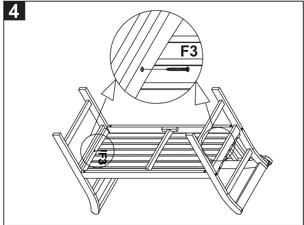
Step 4: use the screw (F3) to fit the seat (D) as shown on the picture and tighten all with a screwdriver.
