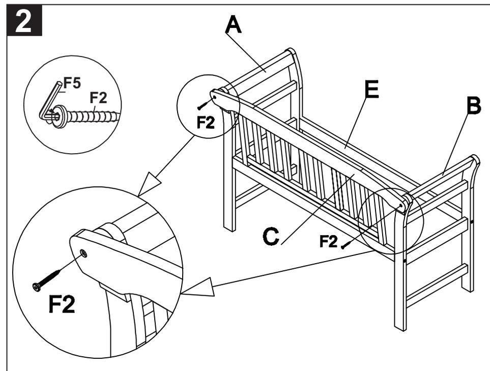
Step 2: use the Allen screw (F2) to fit the back (C) to the side parts (A) and (B) as shown on the picture by using the Allen key (F5).
