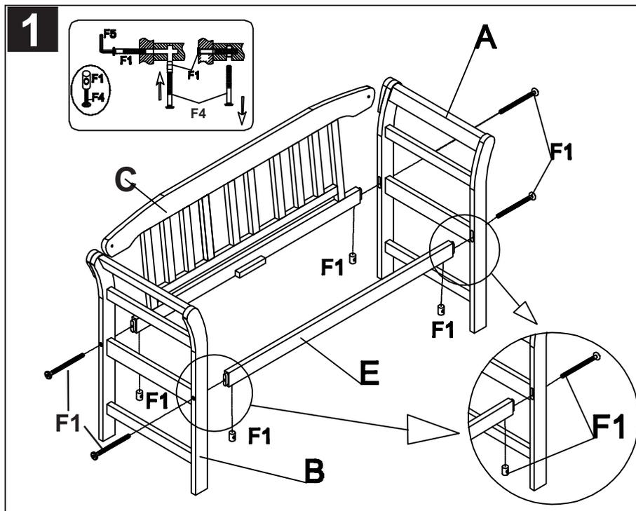
Step 1: attach the left side (A) and the right side (B) to the back (C) and the Support bar (E) as shown on the picture by using the Allen bolts (F1). Tighten all with the Allen key (F5).
