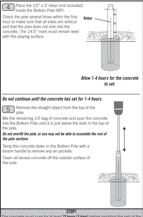
The concrete must cure for at least **72 hours (3 days)** before installing the rest of the system. In humid climates or wet weather, allow additional time for the concrete to cure. Do not proceed until the curing process is complete.
